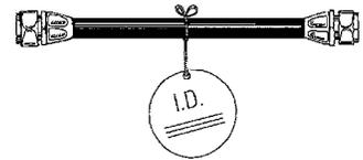
To prevent misapplication, unmarked hose assemblies should not be used unless they can positively be identified.
