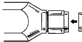
When stored, ends of hose and end fittings should be capped to prevent filtering of dirt and dust into the hose and fittings.
