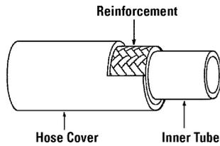
The proper selection of the hose construction to fit the application is of major importance. Generally, hose consists of three basic parts: (1) inner tube; (2) reinforcement; and (3) cover.
