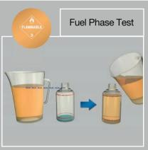
If no water is visible in the sample, fill the bottle to the top line with fuel
