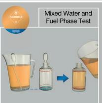
Use pipette to collect free water and put into bottle. If water does not reach lower line, fill to top line with fuel from the same sample
