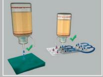
Allow 3 drops to spill onto a tissue to clear the dropper then carefully allow 4 drops of blue fluid into each sample well ensuring no spillage into the viewing window
