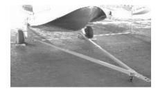
Model TR-PC towbar. This towbar is designed for the Pilatus PC-12 as an easy fold up, carry along, or for everyday ramp use.
