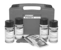
**SK-816 general purpose kit, 16 oz.** Spotcheck visible penetrant kits quickly locate surface cracks. Easy to transport for field inspections. No UV light required because of vivid red color. Includes SKL-SP1 penetrant, SKC-S cleaner and SKD-S2 developer.
