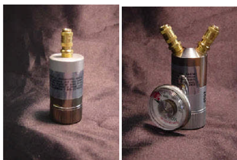
400R1 400R2 400 Series Regulators provide 50-60 liters per minute 25 PSI. Regulator threads are CGA 540.
